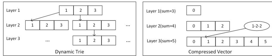
Fig. 3. An Example to illustrate Dynamic Trie and Compressed Vector
