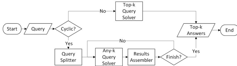
Fig. 2. The Working Process of gTop
